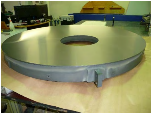
Figure 12. Ready-to-polish M1 FM blank, front face
