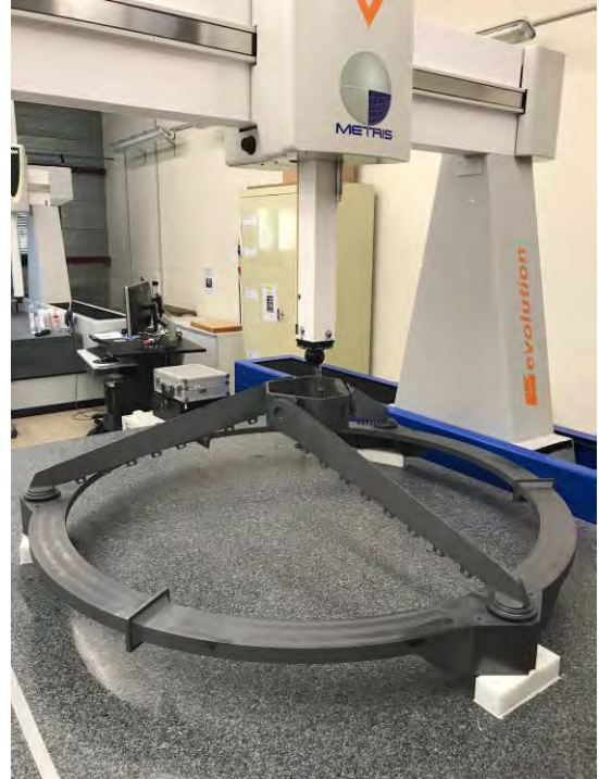
Figure 17. CMM measurement of the spider
